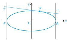
The two tangents drawn at the ends of the major axis are x = a and x = -a
