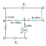
Current through  $R_2 = 20$  mA towards left Applying KVL in loop BGFE  $E_2 = (I + 0.05) 100 + (0.05)20 = 4 \text{ volts}$
