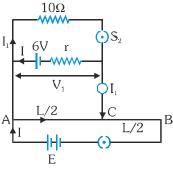
$$V_1 = \frac{E}{R} \times \frac{R}{L} \times \frac{5L}{12} = \frac{5E}{12} = \frac{5 \times 12}{12} = 5V$$
