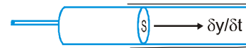
The motion of a piston or Longitudinal pulse, produces an excess pressure p on one side of an element of air. The speed of the element is \delta s/\delta t
