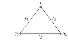
$$U = \frac{1}{4\pi \, \varepsilon_0} \cdot \left[ \frac{q_1 q_2}{r_1} + \frac{q_2 q_3}{r_2} + \frac{q_3 q_1}{r_3} \right]$$
