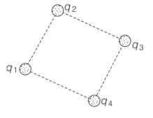
$$U = \frac{1}{4\pi\varepsilon_0} \left[ \frac{q_4 q_3}{r_{43}} + \frac{q_4 q_2}{r_{42}} + \frac{q_4 q_1}{r_{41}} + \frac{q_3 q_2}{r_{32}} + \frac{q_3 q_1}{r_{31}} + \frac{q_2 q_1}{r_{21}} \right]$$
