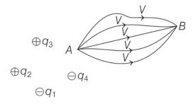
If  $V_A$  and  $V_B$  be the electric potential at point A and B respectively, then  $\Delta V = V_A - V_B$
