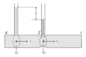
where,  $a_1$  and  $a_2$  are area of cross-sections of tube at broader and narrower part and h is difference of liquid columns in vertical tubes.
