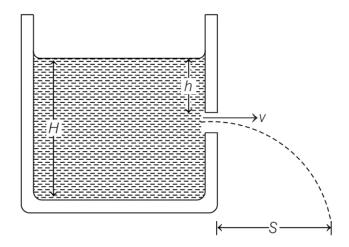
Velocity of efflux,  $v = \sqrt{2gh}$
