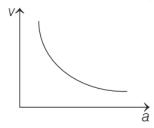
The velocity of liquid is slower where area of cross-section is larger and faster where area of cross-section is smaller.
