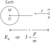
Intensity of gravitational field at a distance r from a body of mass M is given by
