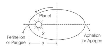
(ii) **Law of area** The radius vector drawn from the sun to a planet sweeps out equal areas in equal intervals of time, i.e. the areal velocity of the planet around the sun is constant.
