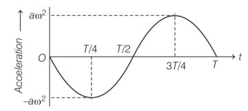
**Note** The acceleration is maximum at a place where the velocity is minimum and *vice-versa*.
