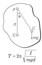
(i) The simple pendulum whose time period is same as that of a physical pendulum is termed as an equivalent simple pendulum.
