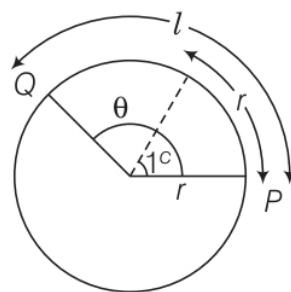
$$\theta = \frac{l}{r} = \frac{\text{Length of arc}}{\text{Radius}} \text{ or } l = r\theta$$
