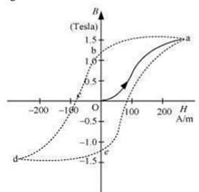
(a) It can be observed from the given curve that magnetization persists even when the external field is removed. This reflects the irreversibility of a ferromagnet.
