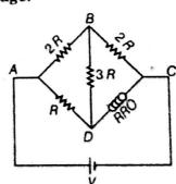
(ii) Calculate the value of R in the balance condition of the Wheatstone
