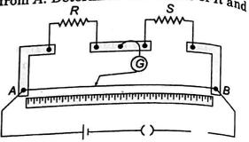
32. In a meter bridge, the null point is found at a distance of  $l_1$  cm from A. If a resistance of  $X_{is}$ connected in parallel with S, then null point occurs at a distance  $l_2$  cm from A. Obtain the formula for X in terms of  $l_1$ ,  $l_2$  and S.
