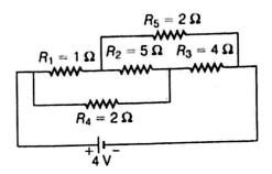
**19.** In the given circuit, assuming point A to be at zero potential, use Kirchhoff's rules to determine the potential at point B.
