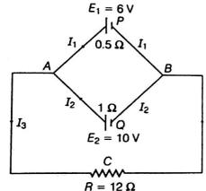
**33.** State Kirchhoff's rules. Apply these rules to the loops PRSP and PRQP to write the expressions for the currents  $I_1$ ,  $I_2$  and  $I_3$  in given circuit.
