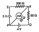
18. Calculate the current drawn from the battery in the given network.
