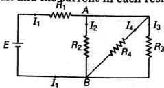
**31.** State Kirchhoff's rules. Use these rules to write the expressions for the currents  $I_1$ ,  $I_2$  and  $I_3$  in the circuit diagram shown in figure below.
