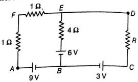
29. Calculate the value of the resistance R in the circuit shown in the figure, so that the current in the circuit is 0.2A. What would be the potential difference between points A and B?
