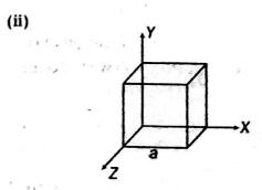
Since, the electric field has only x component, for faces normal to X - direction, the angle between E and  $\Delta S$  is  $\pm \pi/2$ . Therefore, the flux is separately zero for each of the cube except the surface perpendicular to X-axis.
