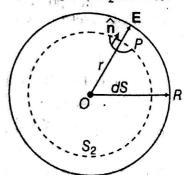
The electric flux through the Gaussian surface, as calculated in Eq. (i), i.e.  $E \times 4\pi r^2$ . As, charge inside a spherical shell is zero, the Gaussian surface encloses no charge. The Gauss' theorem gives
