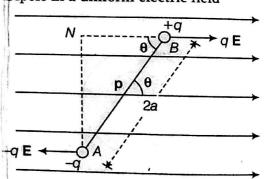
According to the figure, if we consider an electric dipole consisting of charges -q and +q and of length 2a placed in a uniform electric field **E** making an angle  $\theta$  with electric field, then force exerted on charge -q at A = -q **E** (opposite to **E**)
