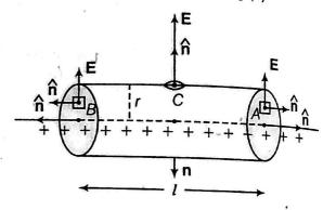
From symmetry, the electric field is everywhere radial in the plane cutting the wire normally and its magnitude only depends on the radial distance (r).
