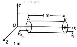
As the electric field is only along the X-axis, so flux will pass only through the cross-section of the cylinder.
