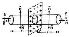
Flux through the flat surfaces = EA + EA = 2EAThe total electric flux over the entire surface of cylinder
