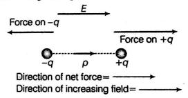
(b) E is increasing anti-parallel to p. So, the torque still remains zero but the net force on the dipole will be in the direction of increasing electric field which is opposite to the dipole moment, hence it will have linear motion opposite to the dipole moment.
