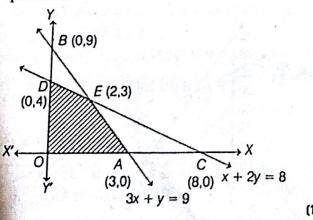
Thus, the shaded region in figure is the feasible region of the LPP. The coordinates of the corner points of this region are O(0, 0), A(3, 0), E(2, 3) and D(0, 4), where the point E(2, 3) is obtained by solving 3x + y = 9 and x + 2y = 8 simultaneously (1) The value of the objective function P = 40x + 50yat the corner points of the feasible region are given in the following table:
