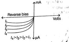
3. The graph shown in the figure represents a plot of current versus voltage for a given semiconductor. Identify the region, if any over which the semiconductor has a negative resistance.
