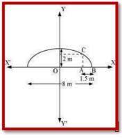
The equation of the semi-ellipse will be of the form  $\frac{x^2}{a^2} + \frac{y^2}{b^2} = 1$ ,  $y \ge 0$  where *a* is the semi-major axis
