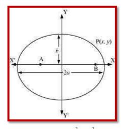
The equation of the ellipse will be of the form  $\frac{x^2}{a^2} + \frac{y^2}{b^2} = 1$  where *a* is the semi-major axis Accordingly,  $2a = 10 \Rightarrow a = 5$
