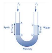
Height of the spirit column,  $h_1 = 12.5 \text{ cm} = 0.125 \text{ m}$ Height of the water column,  $h_2 = 10 \text{ cm} = 0.1 \text{ m}$
