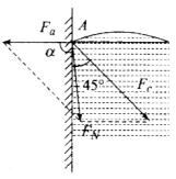
According to the question, the observed meniscus of liquid in a capillary tube is of convex upward which is only possible when angle of contact is obtuse. It is so when one end of glass capillary tube is immersed in a trough of mercury. Hence, the combination will be of mercury-glass (140°) as shown in the figure.
