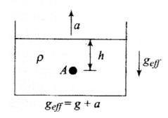
Free surface remains horizontal. Pressure at every point increases. At the point A, P=  $\rho(\text{g}+\text{a})\text{h}$
