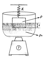
**Important point:** If the scale is not adjusted to zero as said earlier, reading on the scale will be different. Then weight of vessel and weight of water is also added in the reading.
