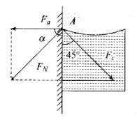
i.e., the resultant force directed outside the liquid. Hence the liquid meniscus must be concave upward.
