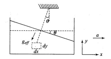
Every fluid element attains an equilibrium position under the action of gravity and pseudo force. The free surface of the liquid orients itself perpendicular to the direction of net effective gravity.
