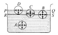
Key concept: To understand the concept of tension acting on the free surface of a liquid, let us consider four liquid molecules like A, B, C and D. Their sphere of influence are shown in the figure.
