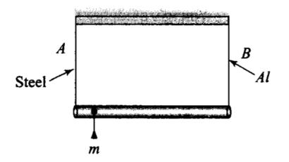
**Sol:** (b, d) According to the diagram a massless rod is suspended at its two ends by two wires of steel (wire A) and aluminum (wire B) of equal lengths.
