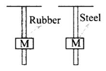
According to the diagram shown below in which a mass AT is attached at the centre of each rod, then both rods will be elongated. But due to different elastic properties of material the steel rod will elongate without making any perceptible change in shape, but the rubber rod will elongate with the shape of the bottom edge tapered to a tip at the centre.
