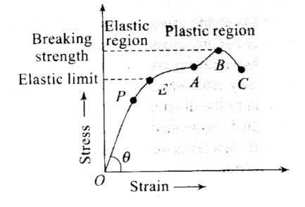
When the strain is small (< 2%) (i.e., in region OP) stress is proportional to strain. This is the region where the so called Hooke's law is obeyed. The point P is called limit of proportionality and slope of line OP gives the Young's modulus Y of the material of the wire. If 6 is the angle of OP from strain axis, then Y= tan  $\theta$ .
