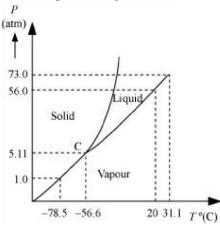
At 1 atm pressure and at  $-60^{\circ}$ C, CO<sub>2</sub> lies to the left of  $-56.6^{\circ}$ C (triple point C). Hence, it lies in the region of vaporous and solid phases.
