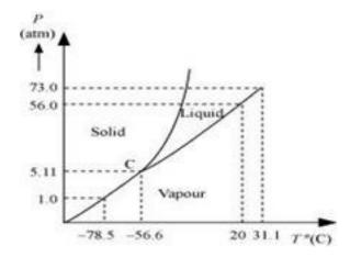
C is the triple point of the  $\mathbf{CO}_2$  phase diagram. This means that at the temperature and pressure corresponding to this point (i.e., at -56.6°C and 5.11 atm), the solid, liquid, and vaporous phases of  $\mathbf{CO}_2$  co-exist in equilibrium.
