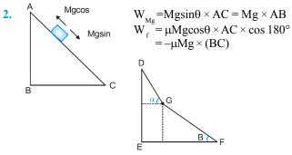
$$\begin{split} W_{Mg} &= Mg(\sin\alpha \times DG + \sin\beta \times GF) = Mg \times DE \\ W_{f} &= -\mu Mg \left( DG \cos\alpha + GF \cos\beta \right) = -\mu Mg(EF) \\ &= -\mu Mg \times BC \qquad (\because BC = EF) \\ From WET, \Delta KE will be same in both cases. \\ \therefore \quad v_{c} &= v_{F} \end{split}$$
